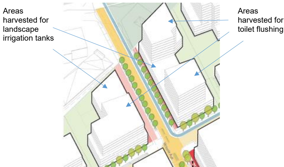
Figure 5-1 Rainwater harvesting arrangement
