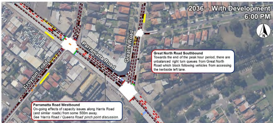
Figure 4-21: Parramatta Road / Great North Road Pinch Point
