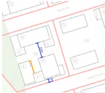
Site 3B as tested, shows the two 15 storey buildings separated by 22m instead of the required 24m. The front setback to Hamilton St was also reduced to 3m instead of 6m to achieve the GFA nominated in the Urban Design Report.
